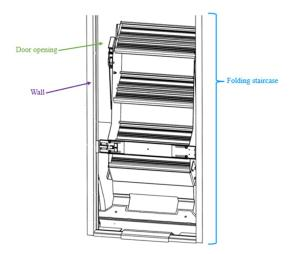
30. The staircase of the Lift Assist Product has a pair of stringers that are spanned by a tread. The staircase has a lower end adapted for contacting the ground surface, and an upper end adapted for abutting the outer wall surface:
