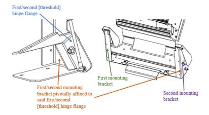
33. The Lift Assist Product includes a hinge with a first mounting bracket pivotally affixed to the first hinge flange and a second mounting bracket pivotably affixed to the second
