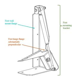
34. The Lift Assist Product includes a second mounting bracket having a second wall mount flange with an inner edge and second hinge flange substantially perpendicular thereto and extending from the second wall mount flange oppositely of the inner edge of the second wall mount flange where the second wall mount flange is adapted for being affixed to the inner wall surface:
