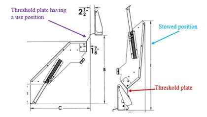
36. The first hinge flange of the threshold plate in the Lift Assist Product is pivotally connected to the first hinge flange of the first mounting bracket, and the second hinge flange of the threshold plate is pivotally connected to the second hinge flange of the second mounting bracket:
